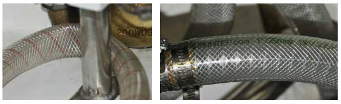
**Left**—While it's commonly installed in onboard water systems, especially by do-it-yourselfers, clear PVC hose is prone to kinking and crushing and should be avoided. **Right**—The exception is kink- and crush-resistant wire-reinforced PVC hose, which is appropriate for pressure and suction applications.
